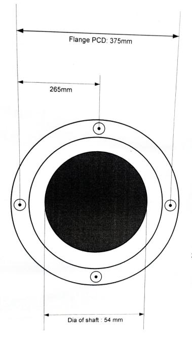
Note: Diameter of Pump-shaft is 54mm
